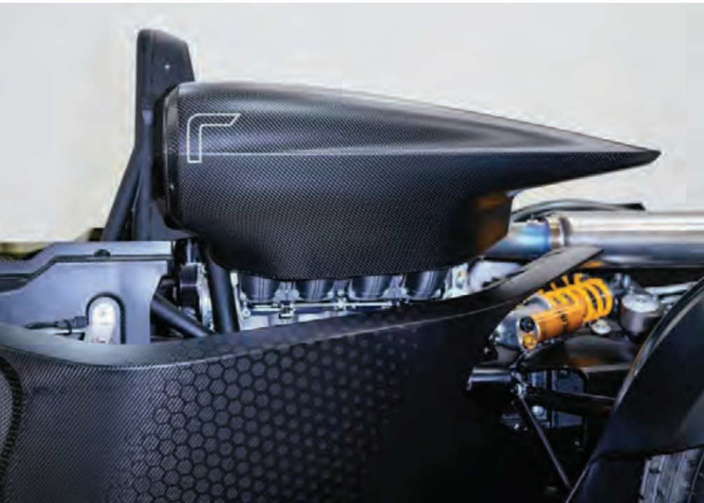
Above and Below: The Mono R continues BAC's tradition of radical innovation in automotive design. It is the first car in the world to incorporate graphene into its carbon fibre chassis; a solution that contributed to nearly 10% weight saving
