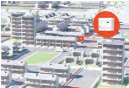
Fifth Generation District Heating with Ambient Shared Borehole Ground Loop Arrays and Kensa Shoebox heat pump.
