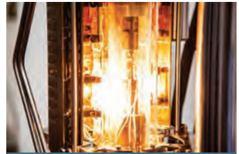
Example of a specimen under test under an extreme environment containing flowing SO 2 and salt.
