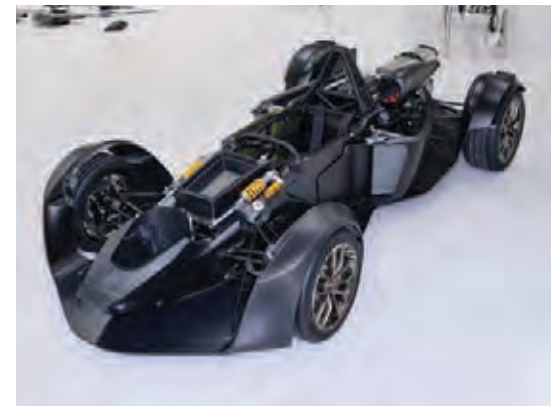
Above and Below: The Mono R continues BAC's tradition of radical innovation in automotive design. It is the first car in the world to incorporate graphene into its carbon fibre chassis; a solution that contributed to nearly 10% weight saving
