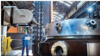
Small modular reactor pressure vessel head being machined at Sheffield Forgemasters.
