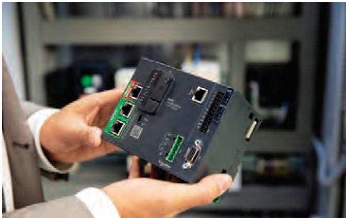
Smart controllers, like the Modicon M262 shown here, are core to smart manufacturing.
