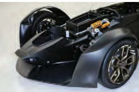
Above and Below: The Mono R continues BAC's tradition of radical innovation in automotive design. It is the first car in the world to incorporate graphene into its carbon fibre chassis; a solution that contributed to nearly 10% weight saving
